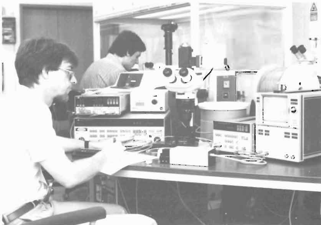
THE HP 8150A OPTICAL SIGNAL SOURCE AND THE HP 8151A OPTICAL PULSE POWER METER PERFORMING A REPEATER MEASUREMENT
